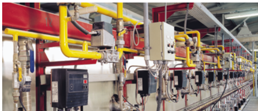
Roller hearth kiln in the ceramics industry
