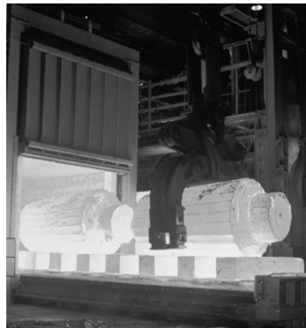
Steel forging furnace
