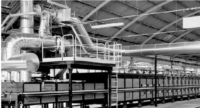
Roller hearth kiln in the ceramics industry
