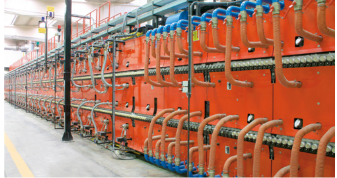
Roller hearth kiln in the ceramics industry
