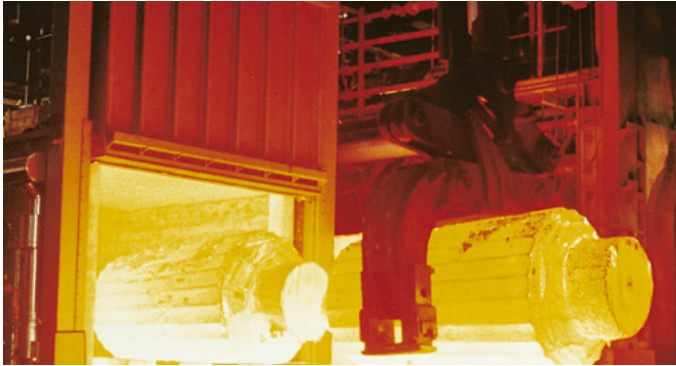
Metallurgical industry: forging furnace
